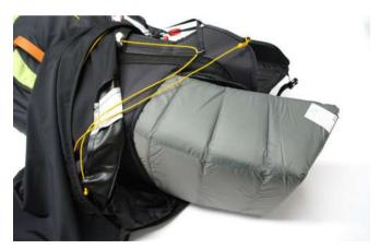
The airfoam pad fills the space between pilot's back and the rescue chute container. It improves the seating comfort while offering additional protection.
