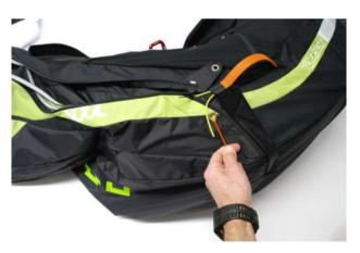
Lead the assist lines through the metal loops of the #3 flap.
