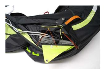
Lead the assist line through the metal eyelet of the #1 flap and secure yellow loop with the longer pin. Put the end of the pin into its pouch. Gently remove the assist line.
